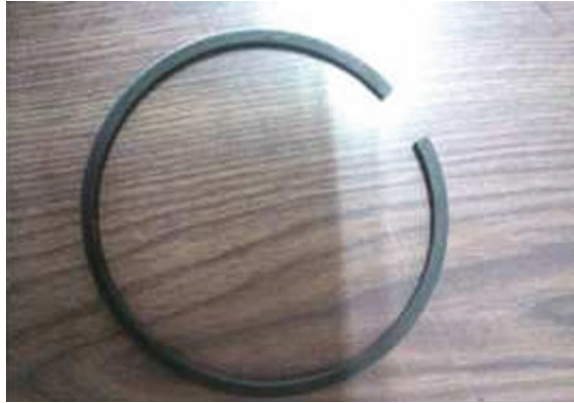
Fig. 2 Moly coated piston ring after honing
